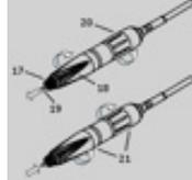
Take the handpiece 21 in your right hand. The motor 20 is thus in the palm of your right hand. Take the crank 18 in your left hand and turn the crank approx. A quarter revolution clockwise until you feel a marked resistance. The chuck is open and the tool can be removed.
