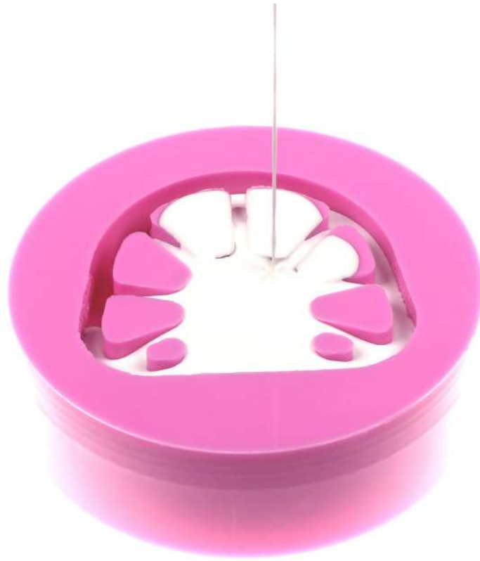
Fig 2 Silicone form filling with plaster
