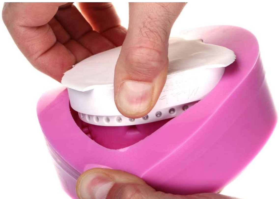
Fig 3 removal of the hardend raw plaster-stabilizer.
