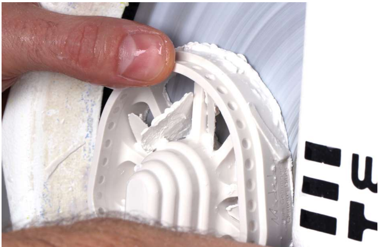
Fig 5 the base is trimmed until the bottom of the flask is fully removed.
