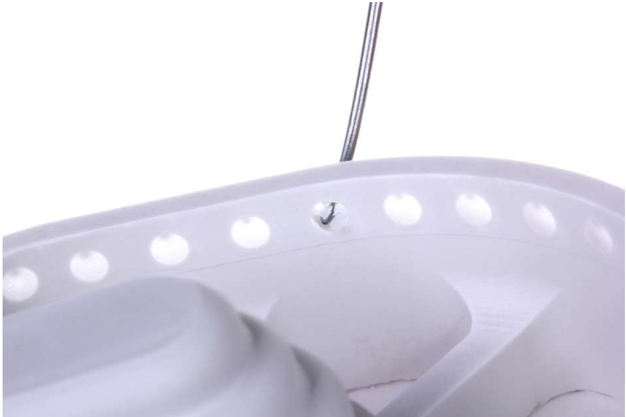
Fig 4 retention windows are pierced with a pointy instrument.
