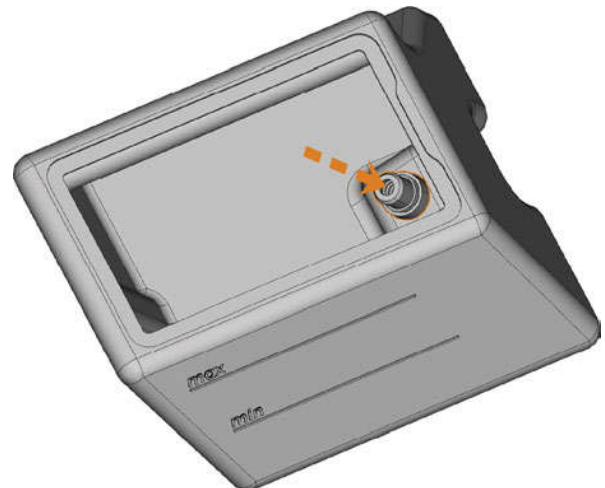
FIG. 91 – PUSHING THE COUPLING OUT OF THE TANK
