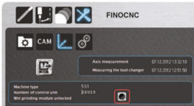
Illustration 40: Part of the machine geometry view Check field for unlocking the wet grinding module marked in red
