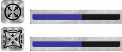
Fig. 18: Top: Value bar and icon for compressed air Bottom: Value bar and icon for the vacuum
