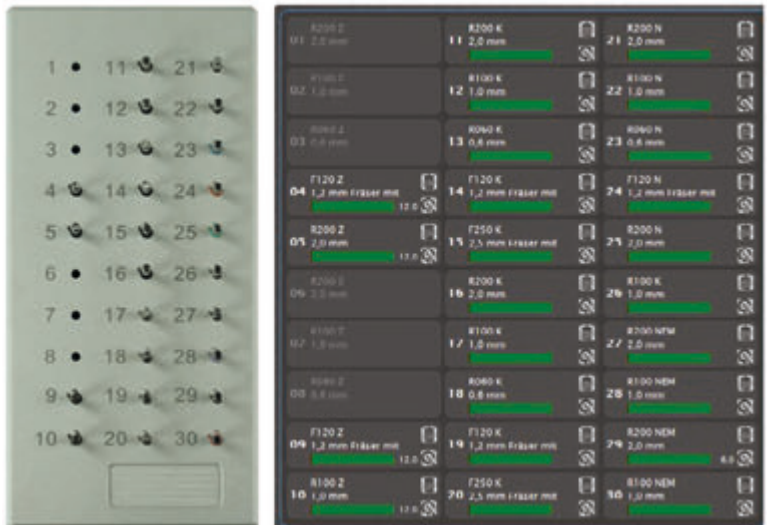
Illustration 45: The tools in the ATB correspond to the tool stock list in FINOCNC
