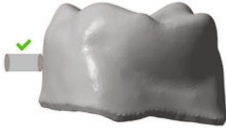
Illustration 29: STL mode of a cap: Suitable surface for a bar
