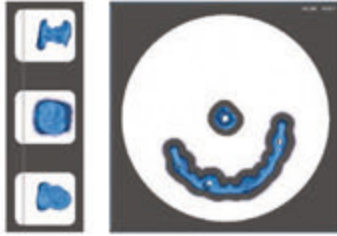
Illustration 18: Two workpiece displays: Grinding block with three objects (left) and blank with two objects (right)
