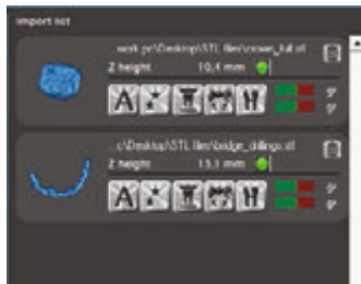
Illustration 17: Import list with two entries. The green icon indicates a sufficient height.
