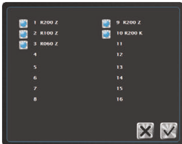
Illustration 50: The window for equipping the tool changer with 5 positions
