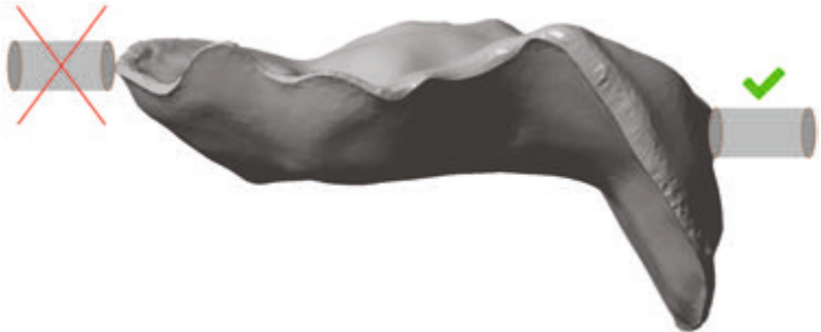
Illustration 27: STL model of an inlay with drawn in bars
