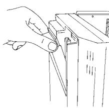
Remove the two fluorescent lamps from their respective holders by pulling in an upward direction.
