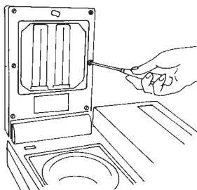
Unscrew the six screws located in the cover plate, and remove both the cover plate and glass plate.
