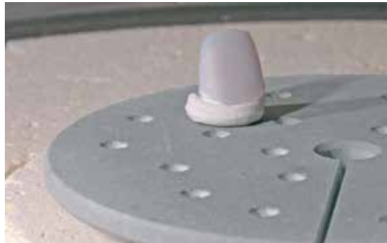
Place the firing tray in the furnace and start Crystallization.
