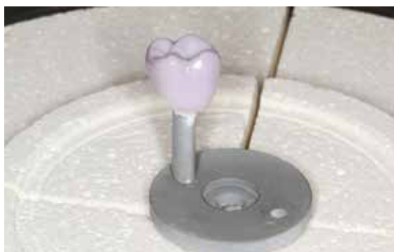
Place the restoration in the centre of the IPS e.max CAD Crystallization Tray and crystallize using the stipulated firing parameters.
