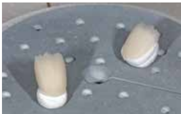
Remove the crystallization tray from the furnace once the Crystallization program has been completed and allow the IPS e.max CAD restoration to cool to room temperature.
