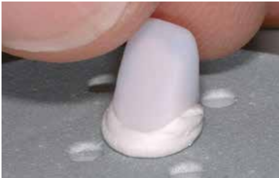
Place the restoration supported with IPS Object Fix Putty or Flow on the IPS e.max CAD Crystallization Tray.
