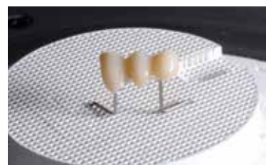
The wash must be fired before the actual layering procedure is started. Place the honey-comb firing tray in the furnace and conduct the Wash firing (foundation) using the stipulated firing parameters.
