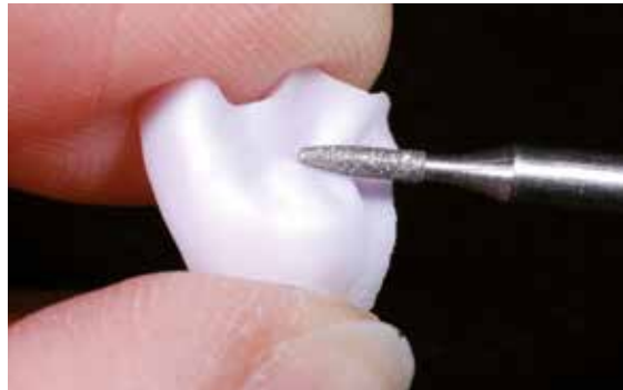
Surface-grind the functional areas in particular with a fine diamond instrument to smooth out the surface structure created by the CAD/CAM procedure.
