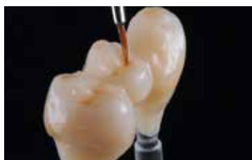
Apply IPS Ivocolor Glaze on the entire bridge and individually characterize the bridge using IPS Ivocolor Shades and Essences.
