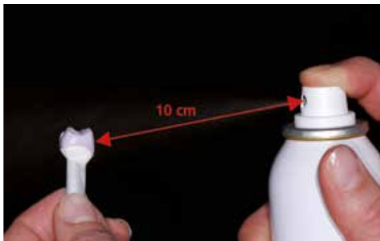
Hold the restoration by the IPS e.max CAD Crystallization Pin.
