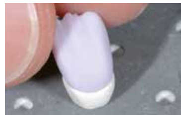
Place the restoration on the IPS e.max CAD Crystallization Tray.
